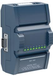
A range of I/O modules are available that have universal inputs and outputs, digital inputs with fast pulse support for use with energy meters and counters, 24VAC triac outputs for use with smaller load applications (up to 1 amp) such as electric fans and motors/actuators and relay outputs for larger load/high power applications such as electric heat and high power actuators.
