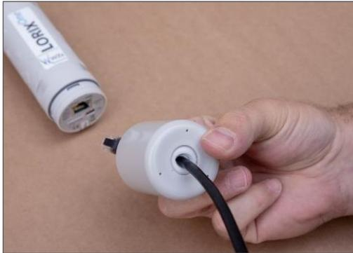
Press the grommet with your finger from inside the cap (left picture) until take it final position (right picture).
