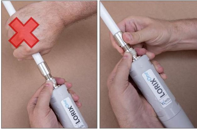
Never turn or use directly the antenna body to screw it on the LORIX One, it could damage or break the antenna.
