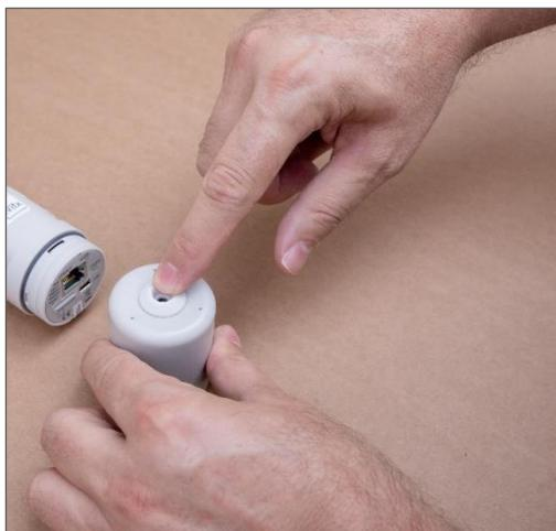
Remove the wire grommet from the cap.
