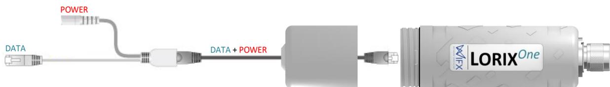
$V_{POE1}$  and  $V_{POE2}$  (in Table 6) represent both power lines of the gateway. Power must be injected in the power input connector using the switching power supply provided with the LORIX One only:
