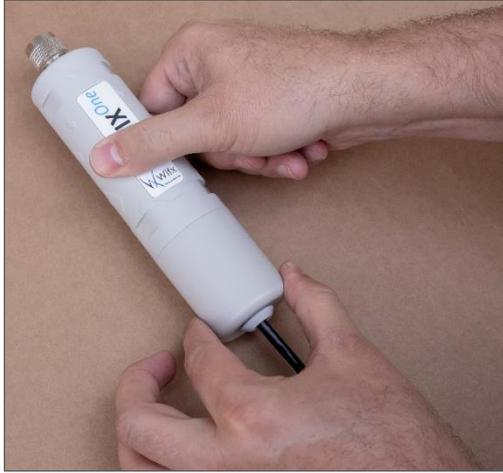
Screw the cap on the body to guarantee as good as possible water and dust protection.
