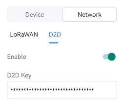
**Step 4:** Enable one of statuses and configure 2-byte hexadecimal Milesight D2D command.
