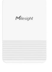
EM320-TH is a simple, compact and powerful LoRaWAN® temperature & humidity sensor. It is equipped with high-precision sensors and IP67 waterproof design, applicable for accurate temperature and humidity data detection in various harsh environments. FDA-approved food-grade material's enclosure and magnet design allow it to be placed in freezers and refrigerators and in contact with food or medicines safely.
