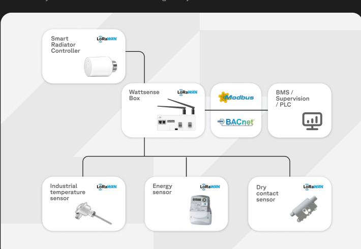
Our IoT solution locally processes raw LoRaWAN frames, decodes them, extracts the data points you selected and sends them directly into a Wattsense Box. The values can be then be easily converted to BACnet IP or Mobus TCP/IP where you define the register adress.
