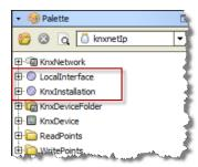
Step 2 If you are not using the **Default IP Multicast Address** of 224.0.23.12, then you should enter it in the **KNX Installation** property.
