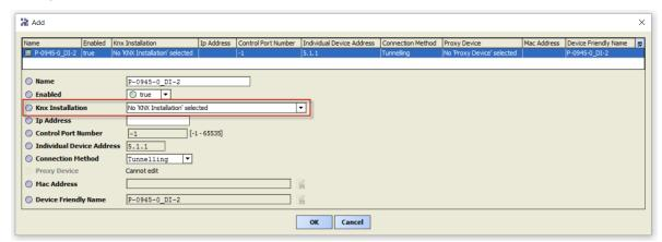
NOTE: When Devices are added by this method, only the **Individual Device Address** property can be reliably derived from the **ETS Project file**. You will need to configure the **Knx Installation** property of each Device. It is **not necessary** to configure the **Ip Address** property because this will be discovered from the Device itself when the **KNX network driver** first tries to connect to the Device, by using its **Individual Device Address**.
