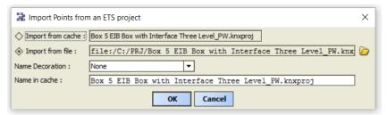
NOTE: The cache retains all the previously loaded ETS project files and you can choose to either use one of these or import a new one. When you choose to **Import from cache** a check is performed to detect changes to the original file since it was last imported into the cache.
