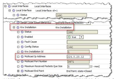
NOTE: If you are using more than one **KNX IP Multicast Address**, you can add additional **KNX Installation** instances from the palette to any **Local Interface**. All the **KNX Installation** instances under a **Local Interface** must have different **KNX IP Multicast Addresses**.
