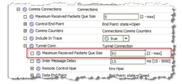
Unlike the **Group Data Operation Queue** (see The 'Read' queue is full, page 58), the necessary size of this queue doesn't depend on the number and frequency of Control Point polling. Instead it depends on how quickly the KNXnet/IP driver can process incoming messages, which in turn depends on the overall CPU usage in the Platform.
