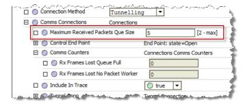
The Maximum Received Packets Que Size (see Knx Device/Comms Connections, page 40) controls the size of the Control End Point's receive queue and it has a default of 5. If this value were too small, there would be an indication of lost frames in the hidden Rx Frames Lost Queue Full Communications Counter (see Knx Device/Comms Connections/Comms Counters, page 42).
