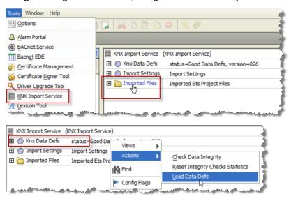
Step 3 Either right click Knx Data Defs and click the Load Data Defs action, or click on Imported Files to load the Ets Project File Import Manager which will examine the new knx\_extra.xml file that was copied into the knx sub-folder of your Niagara installation. You will be presented with a dialogue prompting that there is a newer version available. Click Yes.
