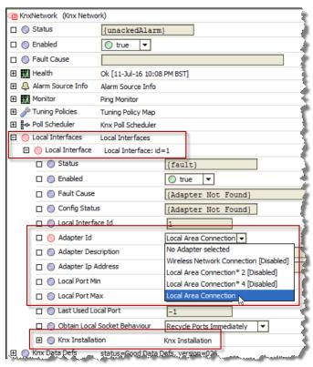
NOTE: Additional **Local Interfaces** can be added from the palette for each of the platform's TCP/ IP Interfaces you wish to use for connection to a **physical KNXnet/IP network**. All the **Local Interfaces** in the station must have different **Adapter Id's**.
