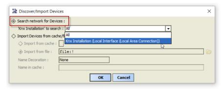
Step 3 Select the **Search network for Devices** option, choose which **Knx Installation** to search and click **OK**. The Discovery process will take about 10 seconds for each **Knx Installation** searched.
