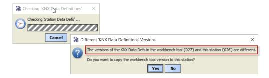
NOTE: There is an issue in v29 of the **KNX Network driver**, whereby after updating the **KNX Data Defs**, examination of the of the Niagara station in the **Property Sheet** of the **KNX Network driver** will still show the older version number in spite of the file being correctly updated. If the station is **Rebooted**, the updated version of the **KNX Data Defs** will be correctly shown.
