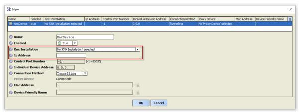
NOTE: When Devices are added by this method, you will need to configure **both** the **Knx Installation** and **Ip Address** properties of each Device. It is **not necessary** to configure the **Individual Device Address** property because this will be discovered from the Device itself when the **KNX network driver** first tries to connect to the Device, by using the **Ip Address**.
