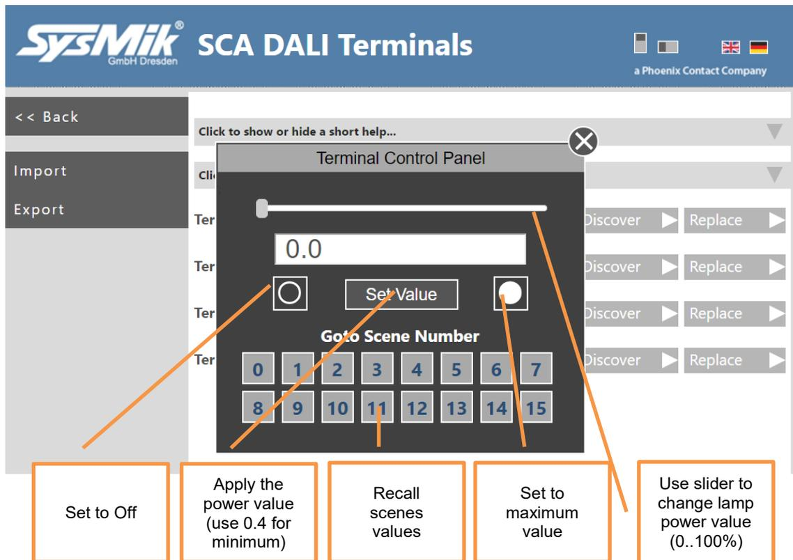
Fig. 2.3.2: Broadcast control panel
