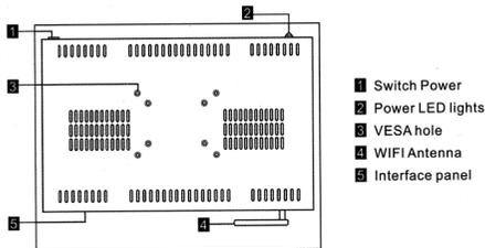
Alternatively, the **VOR-10.1-M-A** can be surface mounted using a suitable VESA bracket. 4x mounting holes are provided in the rear of the screen to secure the bracket.
