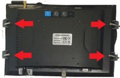
The **VOR-15.6-M-A** is primarily installed in panel mounting mode.
