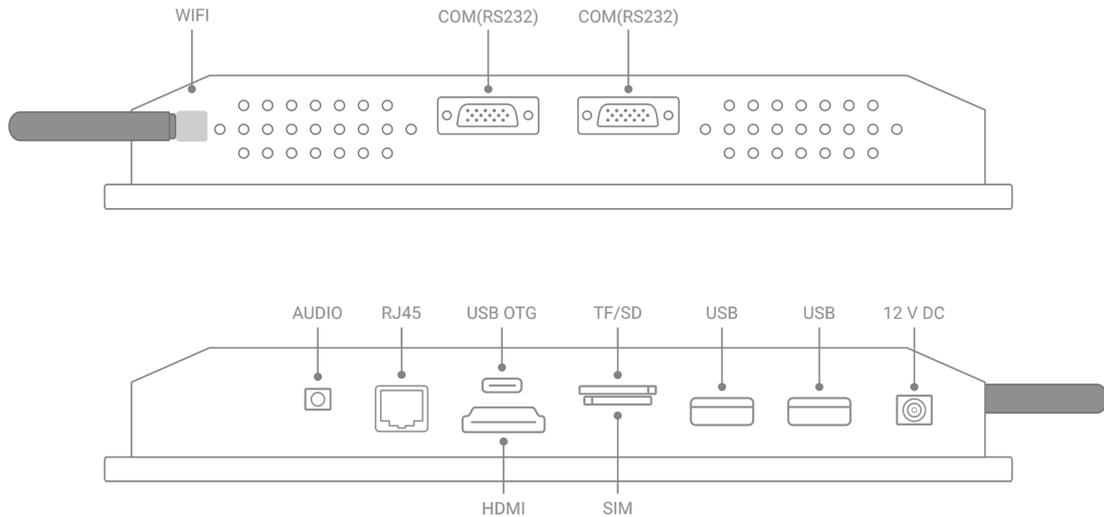
Figure 5. Interfaces of iSMA-D-PA7C-B1
