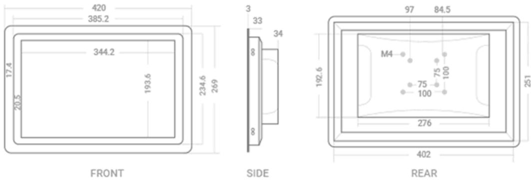
Figure 4. Dimensions of iSMA-D-PA15C-B1
