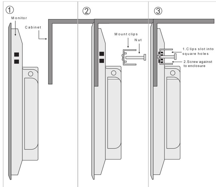
Figure 19. Embed with snap joint installation
