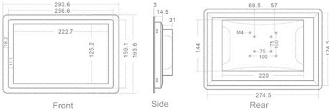
Figure 3. Dimensions of iSMA-D-PA10C-B1
