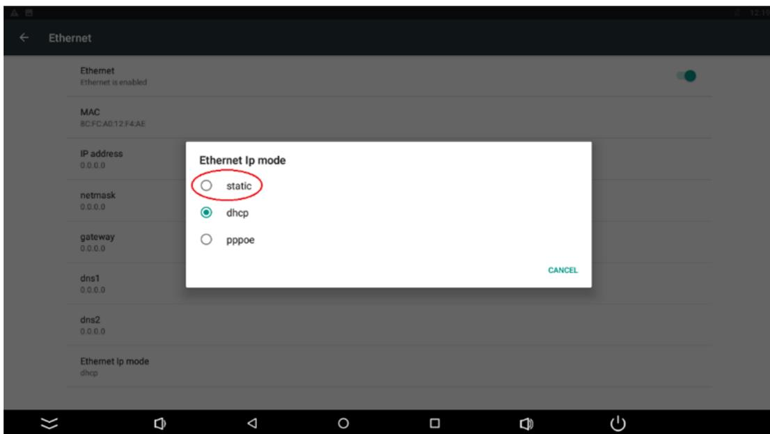
Figure 17. Setting Ethernet IP mode
