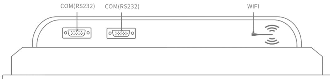
Figure 7. Interfaces of iSMA-D-PA15C-B1
