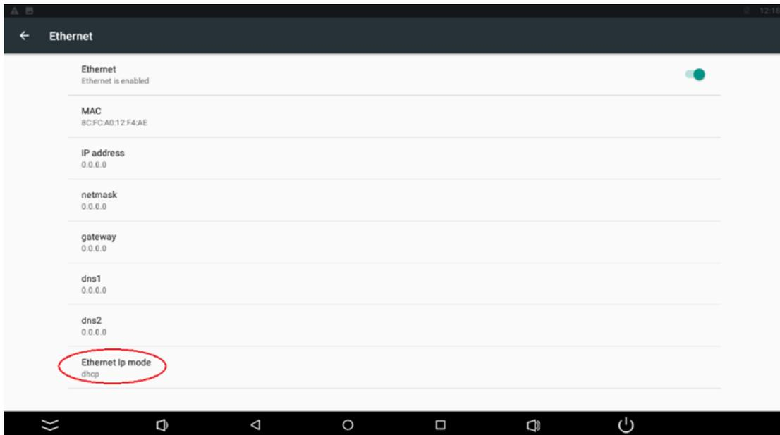
Figure 16. Ethernet IP mode
