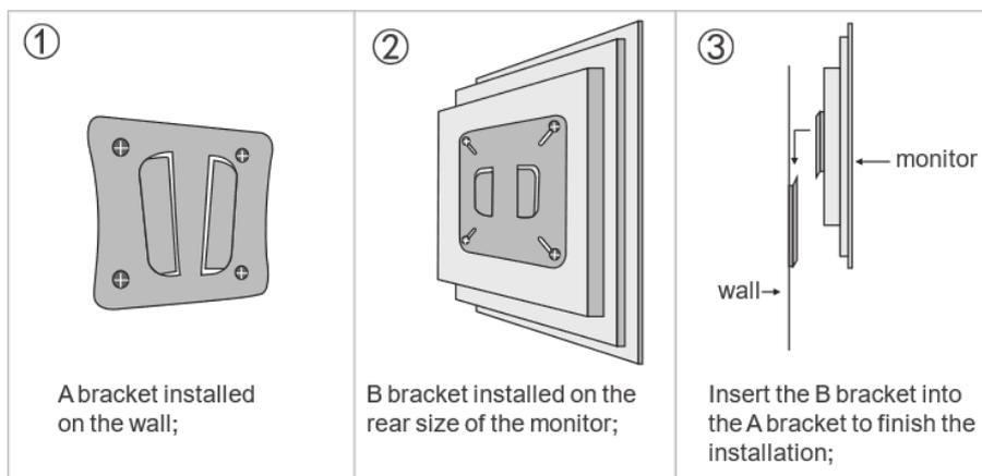
Figure 20. Wall mount installation
