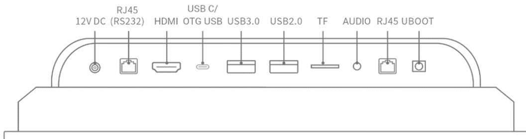
Figure 6. Interfaces of iSMA-D-PA10C-B1
