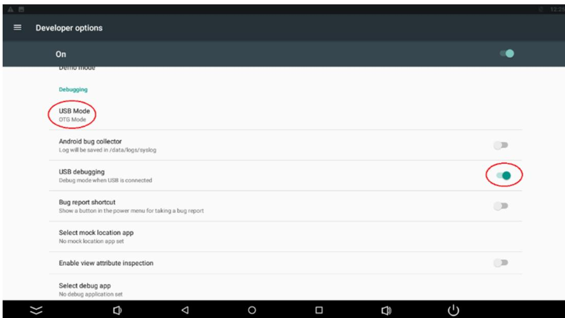
Figure 11. USB mode and USB debugging
