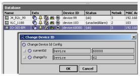
Clicking OK launches a "Change Device Id Job", with an entry in the station's JobService. The job ends with a popup notification that explains whether the Device ID change was successful or not (Figure 3-31).
