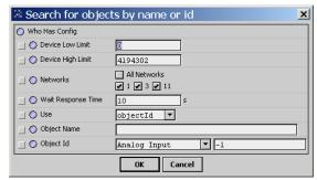
As in the device discover dialog, you can set device low and high limits, as well as select which BACnet networks (by number) receive the Who-Has broadcast (or all networks). When you click **OK**, a Bacnet Who Has job is started, and when the job completes the results (including "I-Have" responses) appear in another popup window, as shown in Figure 3-25.
