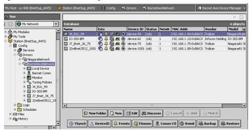
You discover BACnet devices in this view the same as in the **Bacnet Device Manager** view. For details, see "About Bacnet Device Find Parameters" on page 3-27. When doing a discover, the **Add** dialog provides the same parameters for adding BacnetAwsDevices as for BacnetDevices. See "BacnetDevice properties" on page 3-31.
