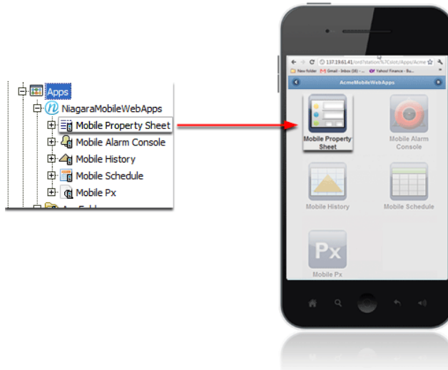
Figure 10. Mobile Property Sheet app in Workbench and in the Mobile Desktop view
