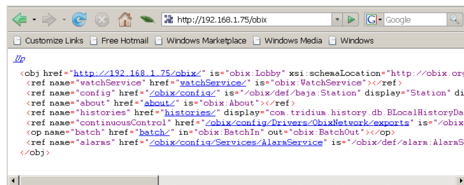
Figure 3-2 Example browser connection to confirm NiagaraAX station oBIX server operation
