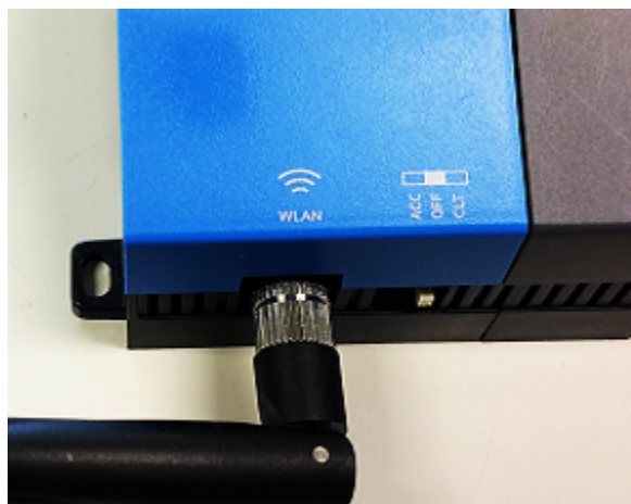
Figure 1. Antenna and switch location on enclosure
