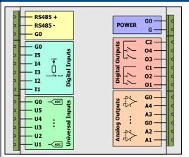
All G0 terminals are connected together internally
