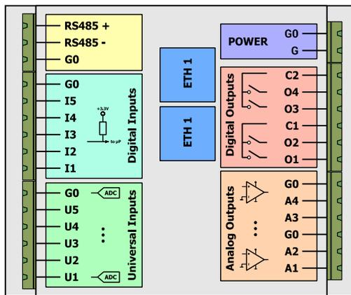
**All G0 terminals are connected together internally**
