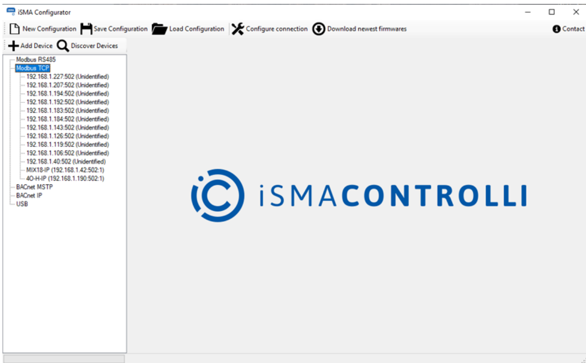
Figure 23. Devices discovered via Modbus TCP/IP
