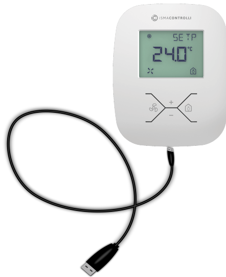
Figure 7. Direct USB connection to an LP panel
