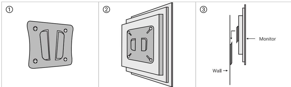
A bracket installed on the wall
