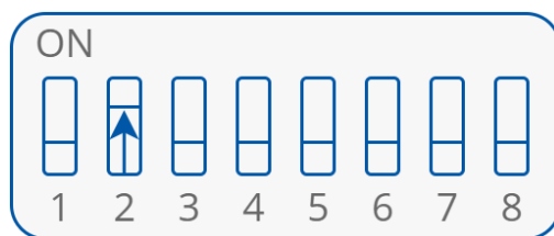
Figure 30. CFG DIP switch configuration for 2-stage heating
