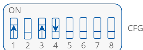
Figure 43. CFG DIP switch configuration for digital control mode
