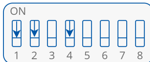
Figure 26. CFG DIP switch configuration in digital control mode
