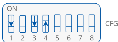
Figure 39. CFG DIP switch configuration for analog control mode
