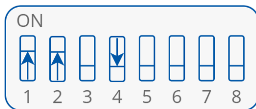
Figure 32. CFG DIP switch configuration for digital control mode
