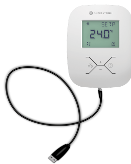
Figure 50. iSMA-B-LP panel USB connection
