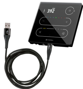
Figure 51. Touch Point panel USB connection
