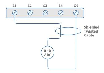
Figure 14. Special inputs in analog mode connection
