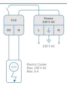
Figure 22. O5 digital output, example of 230 V AC electrical cooler connection (iSMA-B-FCU-HH, iSMA-B-FCU-HL)
