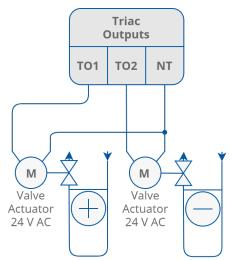
Figure 18. Triac outputs connection
