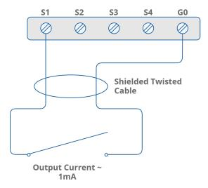
Figure 13. Speical inputs in digital mode connection
