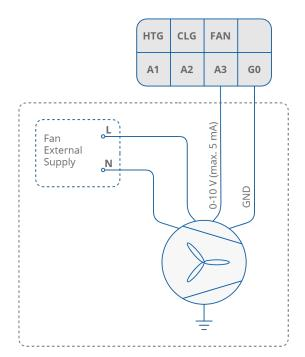
Figure 25. Analog outputs, example of connecting 0-10 V analog fan control
