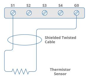
Figure 16. Special inputs in temperature mode connection
