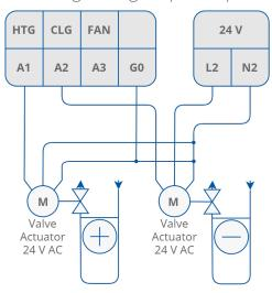
Figure 24. Analog outputs, example of connecting 0-10 V analog valve actuators
