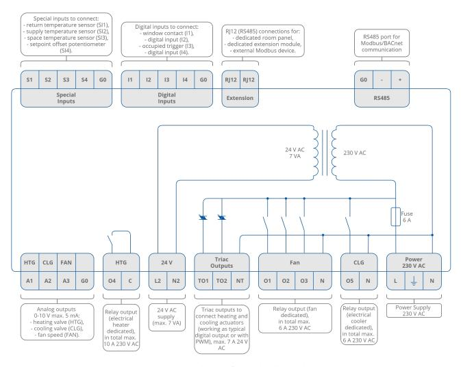
Figure 5. iSMA-B-FCU-HL diagram of terminals and internal connections
