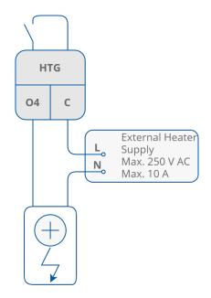
Figure 21. Example of an electrical heater connection
