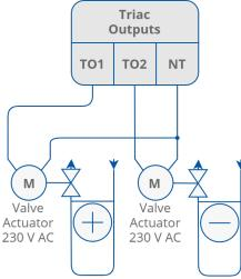
Figure 19. Triac outputs connection
