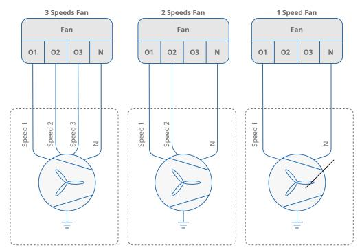
Figure 20. O1-O3 digital outputs, examples of conenctions
