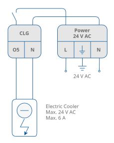
Figure 23. O5 digital output, example of 24 V AC electrical cooler connection (iSMA-B-FCU-LL)
