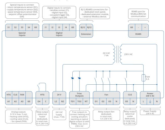
Figure 4. iSMA-B-FCU-HH diagram of terminals and internal connections
