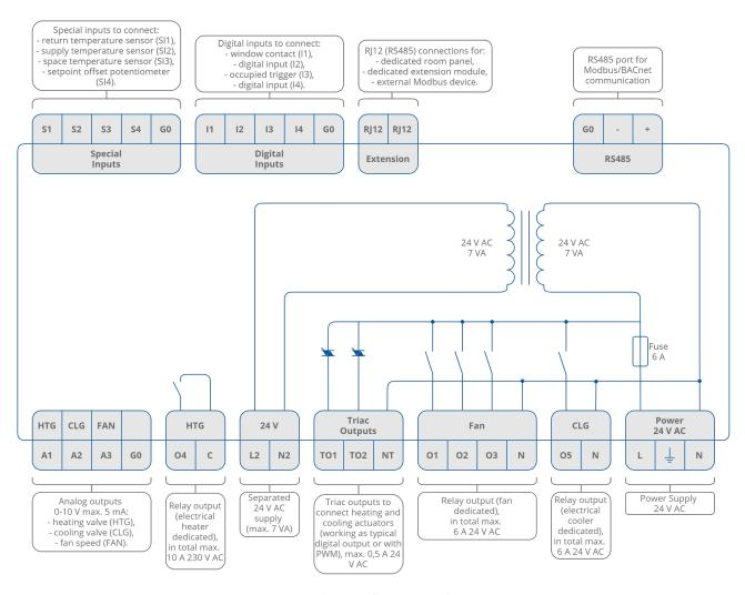
Figure 6. iSMA-B-FCU-LL diagram of terminals and internal connections
