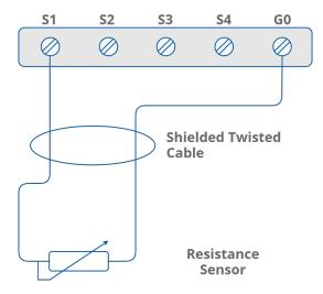
Figure 15. Special inputs in resistance mode connection
